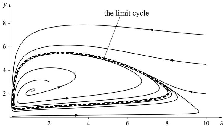
Notice that no matter where we start, the trajectory is apparently always drawn to the closed loop shown in dashes above. This loop is an example of an **attracting limit cycle**. As usual, we could reverse all the arrows in our vector field, in which case this example would be converted to a **repelling limit cycle**.
