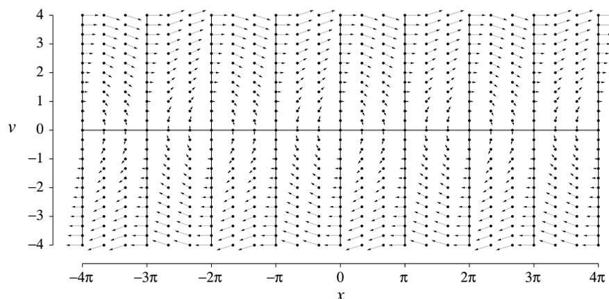
We have included in this diagram the lines where  $v' = 0$  (the vertical lines at every multiple of  $\pi$ ) and the line where  $x' = 0$  (the horizontal line at  $v = 0$ ). Note that the velocity vectors are horizontal on the lines corresponding to  $v' = 0$  and are vertical on the line corresponding to  $x' = 0$ . The points where these two sets of lines intersect—all points of the form  $(k\pi, 0)$  for  $k$  an integer—are the equilibrium points of the system. Let's sketch the phase
