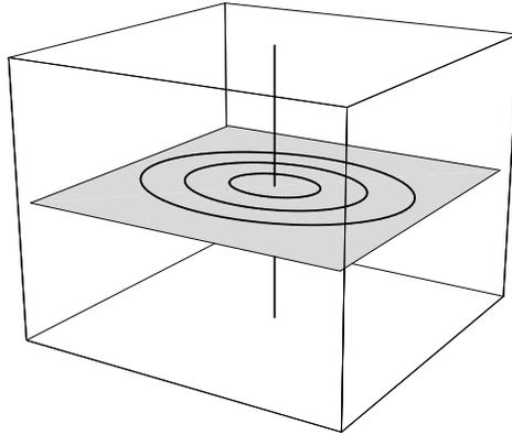
It is worth pointing out that we can represent the two-dimensional systems we’ve been exploring so far in this chapter in three dimensions by introducing a time axis. This has the effect of “unwinding” the trajectories by stretching them out in the  $t$ -direction: closed trajectories become endless coils, equilibrium points become straight lines parallel to the  $t$ -axis, and so on.
